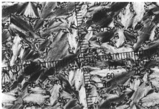
Figure 8. Optical polarization micrograph of PB-F-S6 annealed at 79.8 °C for 2 days.
